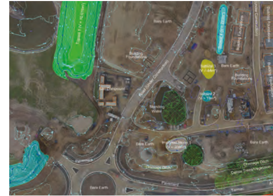
Topographic survey output including stockpile volumetrics
